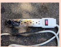
**Space Heaters:** Under the "a picture is worth a thousand words" category, the accompanying photo dramatically reflects what can happen if you plug a space heater into a power strip/extension cord. Don't rely upon the circuit breaker of that < \$20 power strip to trip, if overloaded.
